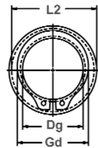
Clearance Diameter & Gaging Diameter Released in Groove.
