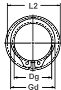
Clearance Diameter & Gaging Diameter Released in Groove.
